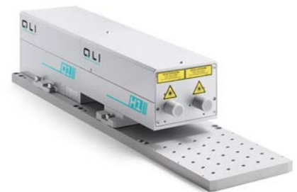
Laser head Q1 with H1 harmonic generator and base plate
